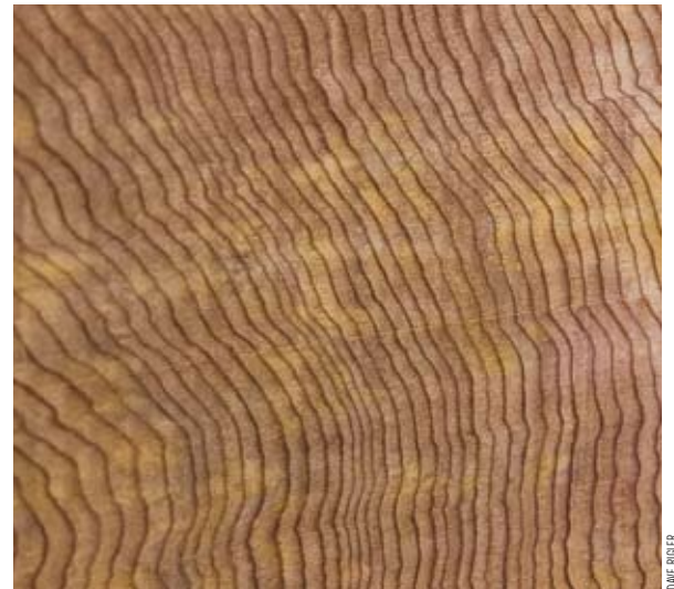
A close-up of the cedar after a similar pass shows slight cutter marks...
