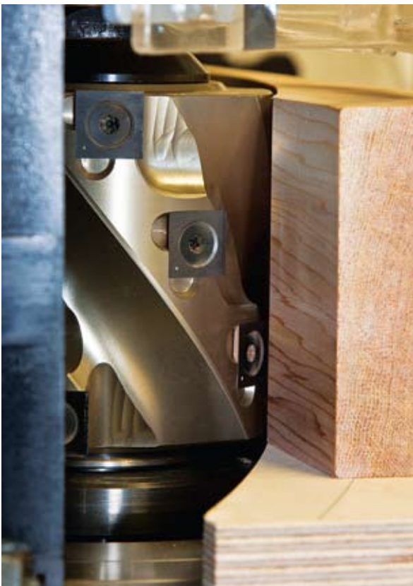
Great results from the spiral cutter right up to the 75mm limit
