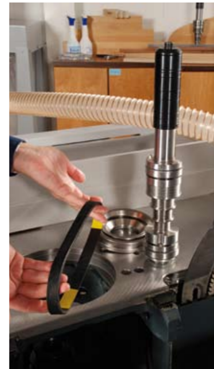
The vertical adjustment on the new machine eliminates misalignment of the fence carrying edge
