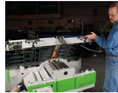
The vertical adjustment on the new machine eliminates misalignment of the fence carrying edge
